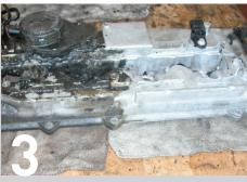
Removed valve cover. Left: untreated. Right cleaned with Cold Spray, LIQUI MOLY Pro-Line Injector and Glow Plug Dismantling Aid and engine wash.
