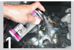
Spray all parts thoroughly with Cold Spray and LIQUI MOLY Pro-Line Injector and Glow Plug Dismantling Aid. Then allow it to work.
