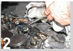
Scrape off and respray several times. Then give the engine a thorough wash.
